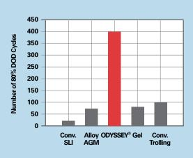
Long Cycle Life ODYSSEY<sup>®</sup> Extreme Series<sup>™</sup> batteries routinely deliver up to 400 deep cycle (80%) discharges.
